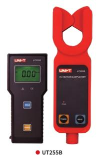
UT255 series high voltage clamp ammeters can measure up to 69kV high voltage line current and leakage current. UT255 comes with an insulation rod, allowing professional users to check status of lightning arresters. The wireless model (UT255B) is also able to wirelessly transmit data in real-time up to 30m range. Its clamp can be easily removed from wire by pressing or pulling back the insulation rod.
