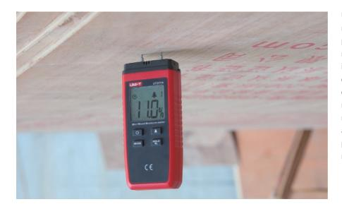
UT377A is a digital meter designed to measure the moisture content of wood, paper, plywood, and other wooden materials. This device classifies wood into four categories based on material density, and applies temperature compensation algorithm to ensure measurement accuracy. UT377A's miniature design, low power consumption, and high precision all make this a great product choice for measuring wood moisture content.
